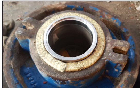
DualPac 2211 Packing installed in the stuffing box. Note the top ring is turned to use the aramid to resist extrusion.
